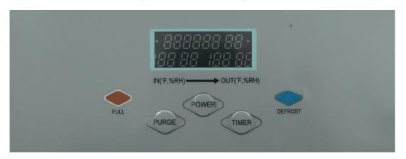
**Power Button:** When the machine is in the standby mode, the display screen will be displayed in low light LED. To start the dehumidifier, press the power button. Concurrently, the display
